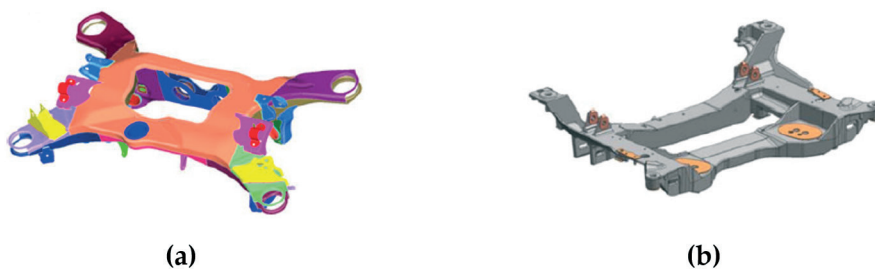
Fig. 2. a) Structure of the rear part of the chassis with 28% less mass compared to the original steel one, b) magnesium motor bed with 35% less mass compared to the original aluminium one [29]
