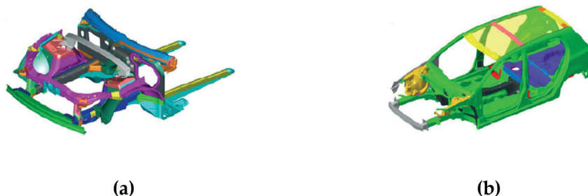
Fig. 3. a) The front end of the vehicle [mostly magnesium] with 45% weight reduction compared to the original version, b) European Union Super Light Vehicle with 35% weight reduction compared to the original version [29]
