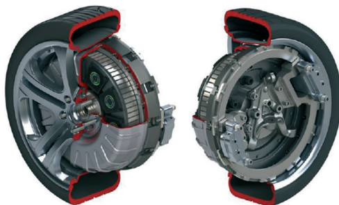
Fig. 10. In-wheel electric motor assembly, Protean/Brabus E-class, front-left corner [38]
