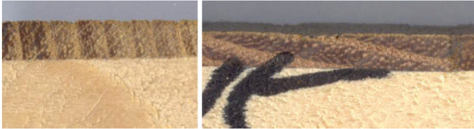
Fig. 10. Cross sections of black locust lamellae, showing surface roughness on the LR (a) and waviness on the LT (b) anatomical planes
