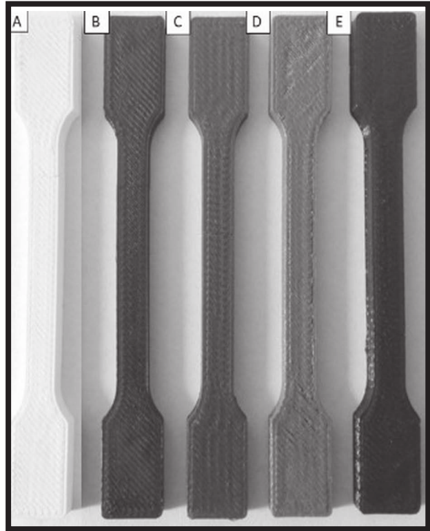
FIG. 12. 3D printed dogbone shape samples: A) PLA, B) PLA/SCF_C, C) PLA/SCF_R, D) PLA/GO, E) PLA/CNT.
