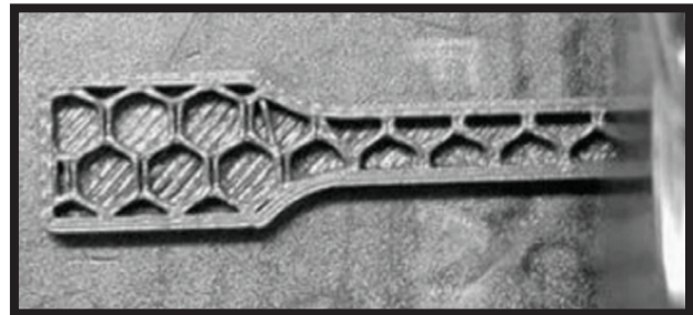
FIG. 13. Hexagonal infill (20%) of the PLA/SCF_R sample.
