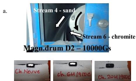
Fig. 2. View of magnetic drum: a – really installation and b – visual neodymium magnet test results of chromite samples subjected to various heat treatments (new chromite and comparably with chromite after two thermal treatment kinds – which is more and more magnetic)
