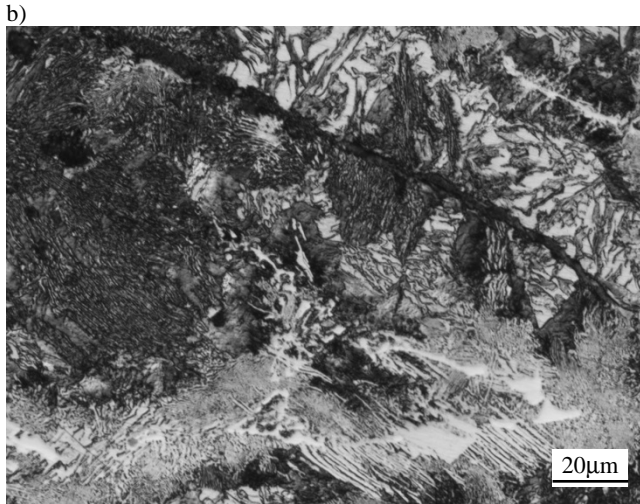
Fig. 4 (a, b). The microstructure of grey cast iron in cellulose profile: flake graphite, pearlite, ausferrite, carbides
