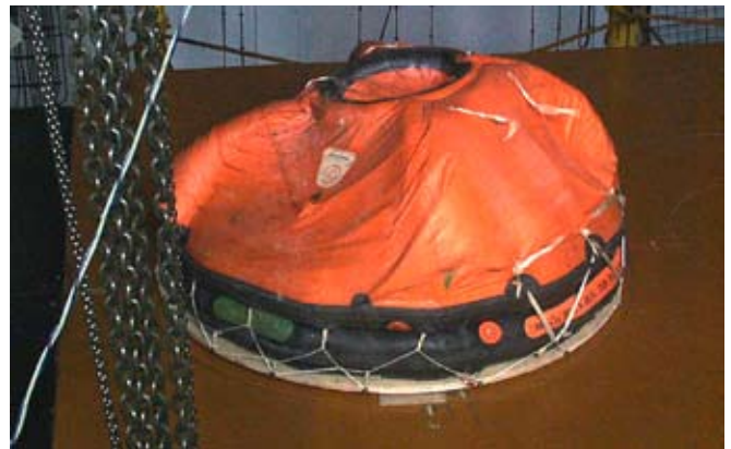
Fig. 6 Investigations of wind pressure force of the life raft conducted at Aerodynamic Laboratory of the Air force Institute in Warsaw.
