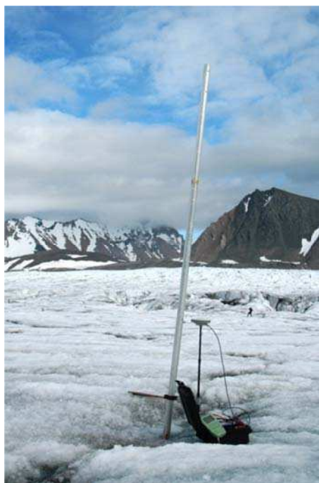
Fig. 9. Position measurement of ablation poles using GPS RTK technique on Hans Glacier (A. Adamek)
