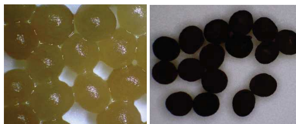
FIG. 1. Microscope images of WPI and ALG microparticles containing active substance: A) swollen microparticles, B) dry microparticles.
