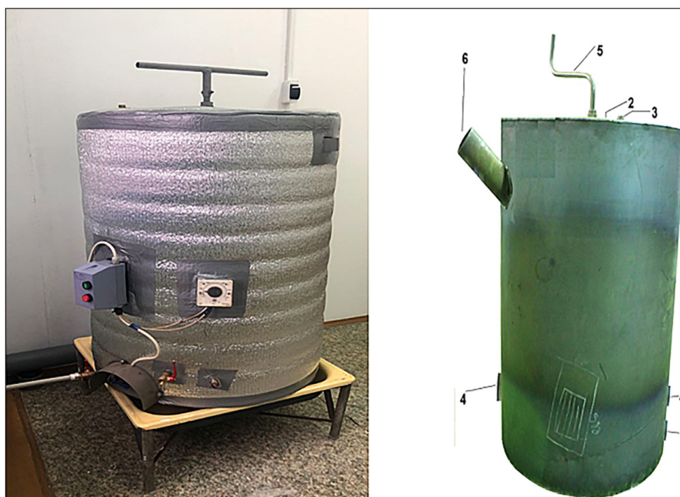
Figure 1. The BUG-R bioreactor, 1 – the heating element for water heating, 2 – the hatch, 3 – the valve for removing the resulting gas, 4 – the hole for draining the substrate and for cleaning and flushing the internal tank of the bioreactor, 5 – the shaft handle, 6 – the hole for loading the substrate
