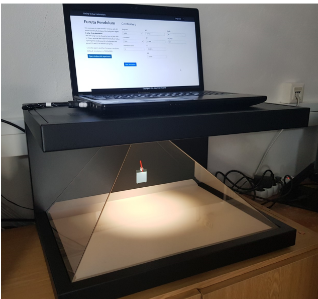
Fig. 10. Dreamoc HD3.2 displaying Furuta pendulum controlled via control interface
