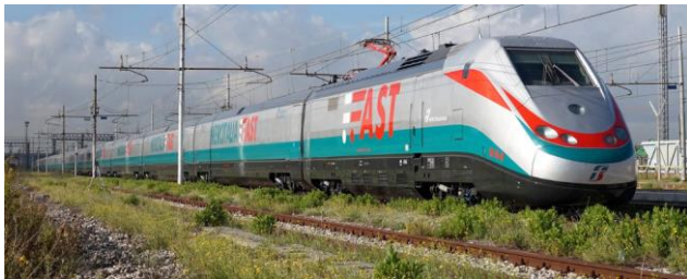
Fig. 18. The Italian high speed freight train ETR M-01 Fast, a modernized version of the ETR 500 vehicle [39]
