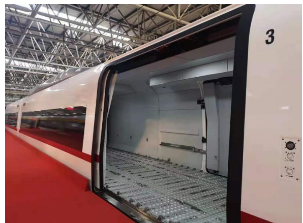
Fig. 27. Loading door – 2.9 m wide [11]
