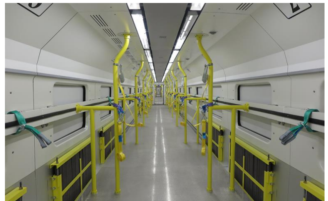
Fig. 20. Freight space in one of the wagons of the ETR M-01 Fast train by Mercitalia [36]
