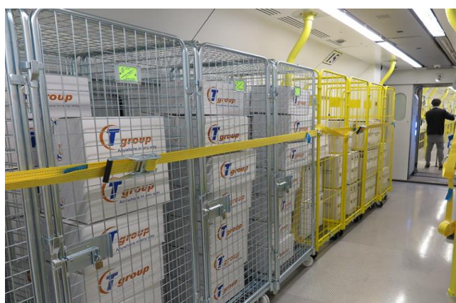
Fig. 23. Containers in the cargo area secured with belts and prepared for transport [36]
