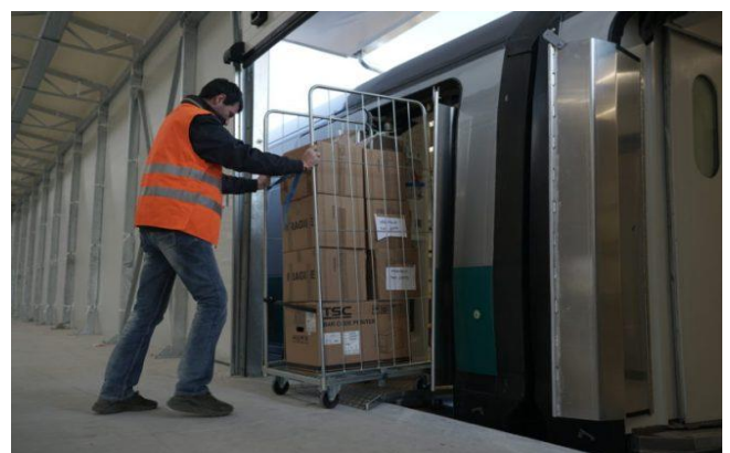
Fig. 21. Loading of containers on wheels to the high speed freight train ETR M-01 Fast [34]
