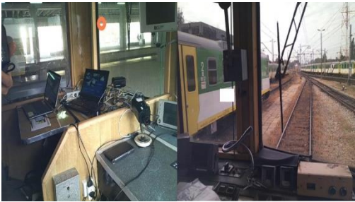
Fig. 5. View of the driver's cab used in the study from the driver's perspective, with the measuring instruments in the background
