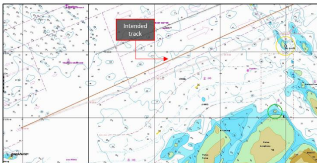
Figure 6. Vessel drift-off and consequential grounding as a result of EPFS failure
