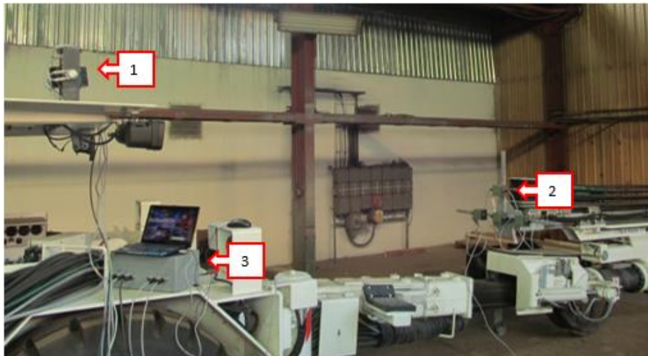
Fig. 5. The face drilling monitoring system installed on the drilling rig, shown during surface tests: 1 - laser beam emitting unit, 2 - photodetector matrices unit, 3 - control system with display
