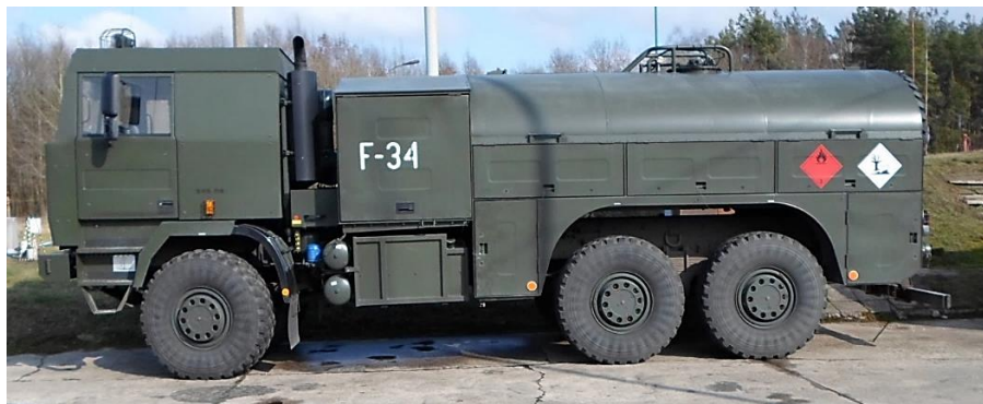
Figure 6. Tanker-dispenser truck with a capacity of 10 \text{ m}^3 (CD-10) on the Jelcz P662 D.34 off-road chassis;
