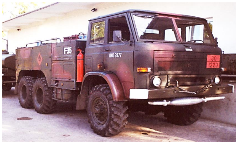
Figure 5. Tanker-dispenser truck with a capacity of 5 m 3 (CD-5) on the 6x6 Star 266 off-road chassis;
