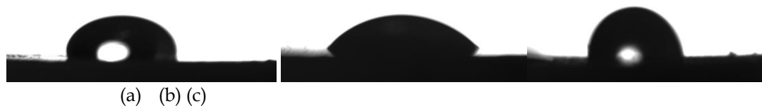
Fig. 14. Contact angles of calcium stearate (a), unmodified calcite (b) and modified calcite (c)
