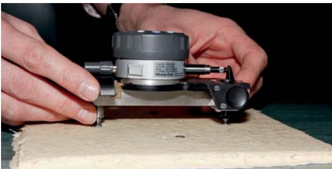
Fig. 5. Extensometer used for length change measurement
