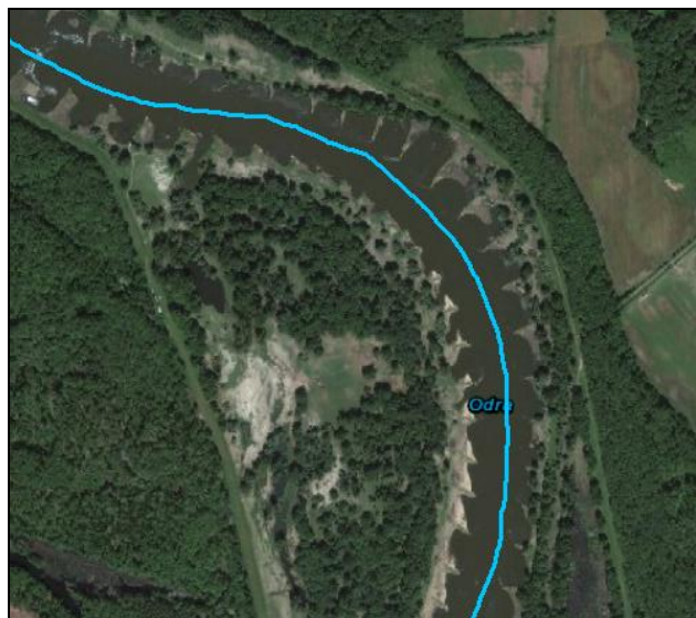
Fig. 5 The position of the GPS RTK receiver placed on the inland vessel when negotiating a bend in the central part of the Odra. Source: [own study using ArcGIS].
