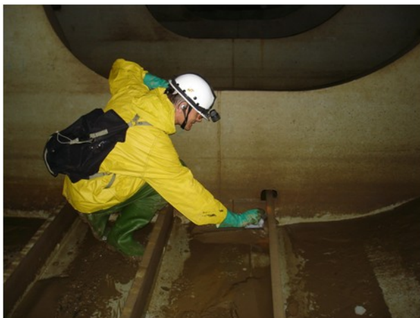
Fig. 3. Sampling of sediment in a ballast tank
