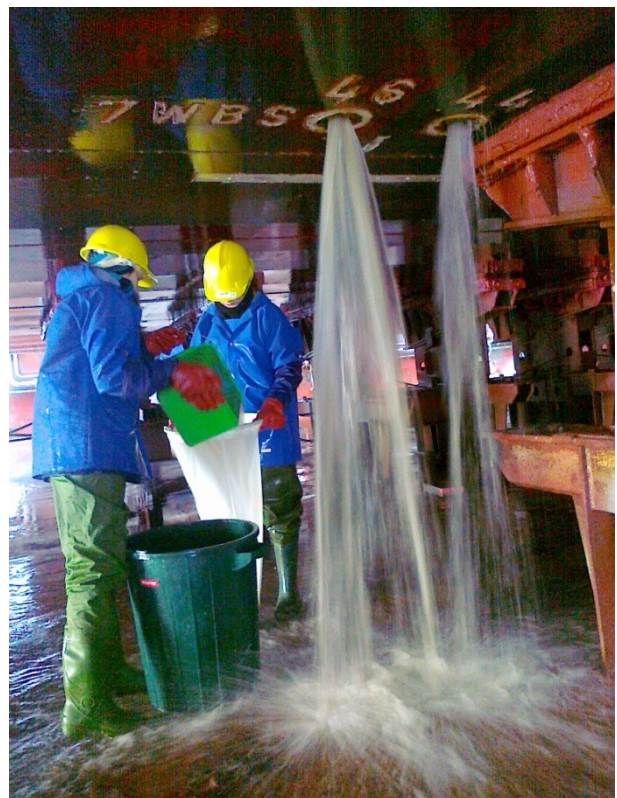
Fig. 2. Sampling of ballast water on the dry dock
