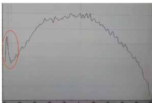
Fig. 2. Thickness cross profile of high-silicon steel strip with the "cat ear" deformation
