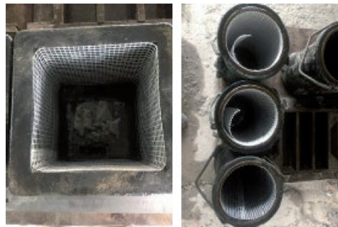
Fig. 1. The micro synthetic fibers were cut and laid according to the dimensions of the moulds
