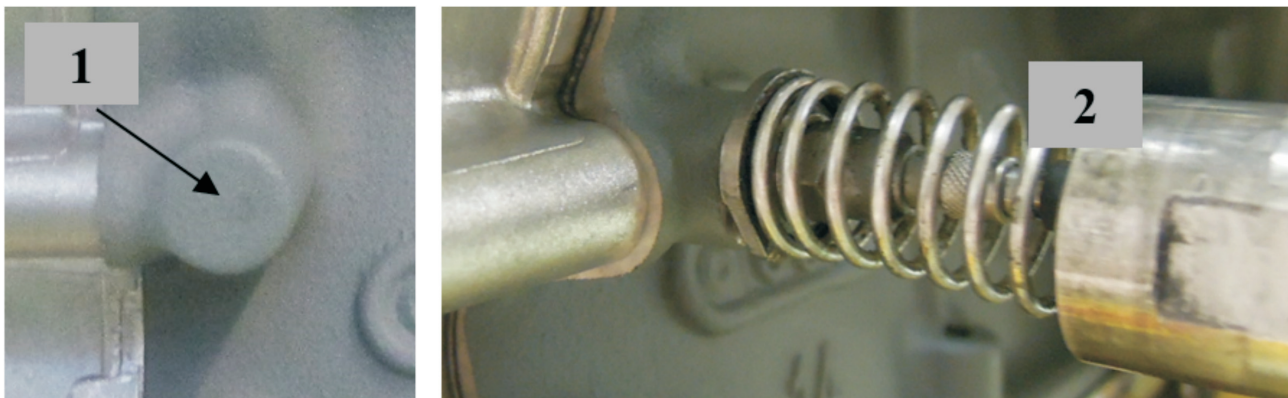
Fig. 2. Attachment of the piezoelectric sensor (measurement of vibrations of the cylinder block): 1 – position of contact of the cylinder block with the sensor, 2 – sensing unit during operation
