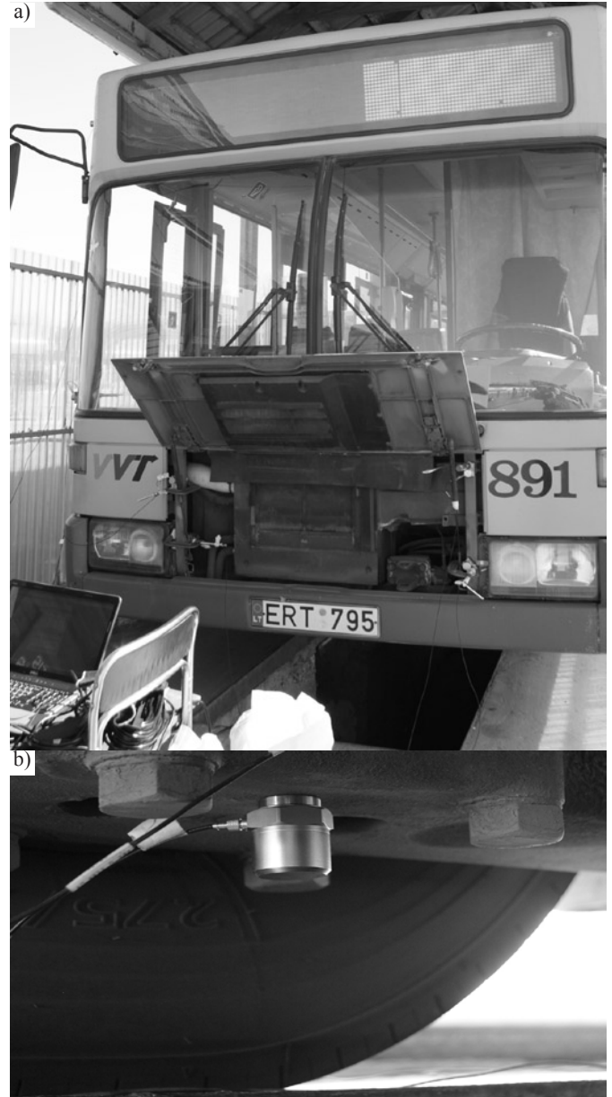
Fig. 1. The measuring equipment of vibration parameters: a) portable measurement data: processing, storage and control equipment „3660-D“ with DELL computer; b) accelerometer 8344.
