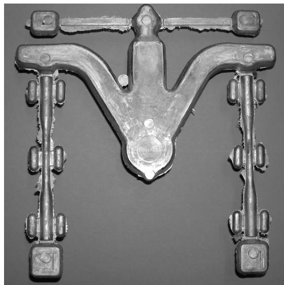
Fig. 1. Macrograph of AME505 experimental magnesium alloy cast fabricated by IDRA-380 cold-chamber die-casting
