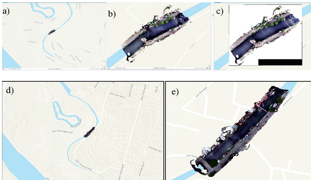
Figure 4. a) Survey location 10m altitude, b) Mosaic data from 561 images into seven raster data, c) Mosaic seven images into 1 raster data, d) Survey location 15 altitude, e) Mosaic data from 351 images into one raster data
