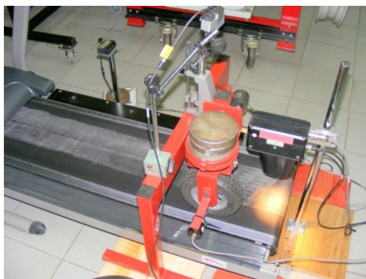
Fig. 4. The test bench for measuring the tire cornering stiffness
