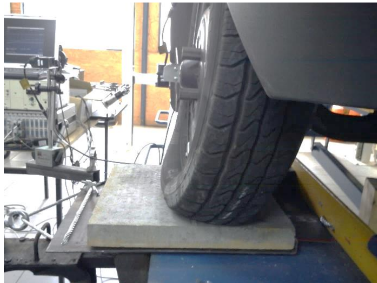
Fig. 2. Measurement of tires stiffness – 185R15C
