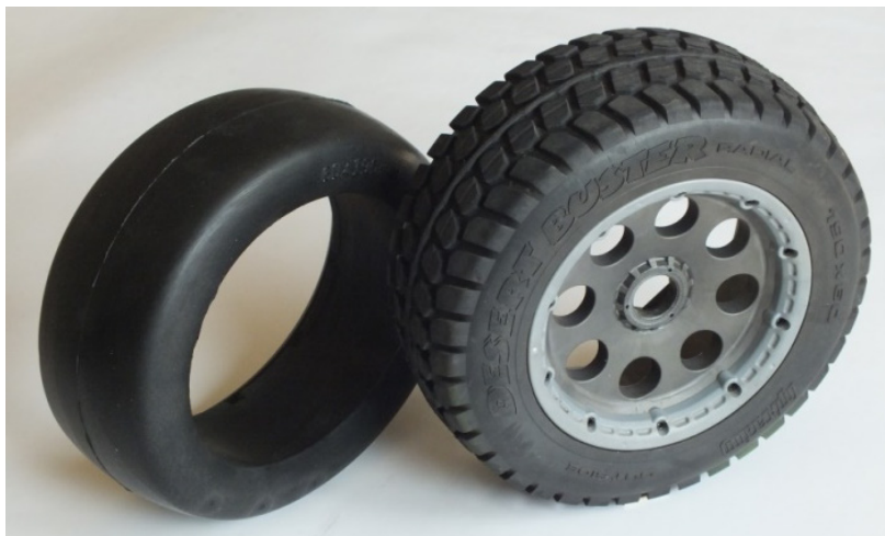
Fig. 1. The tire with a polyurethane insert used in a vehicle made in smaller scale
