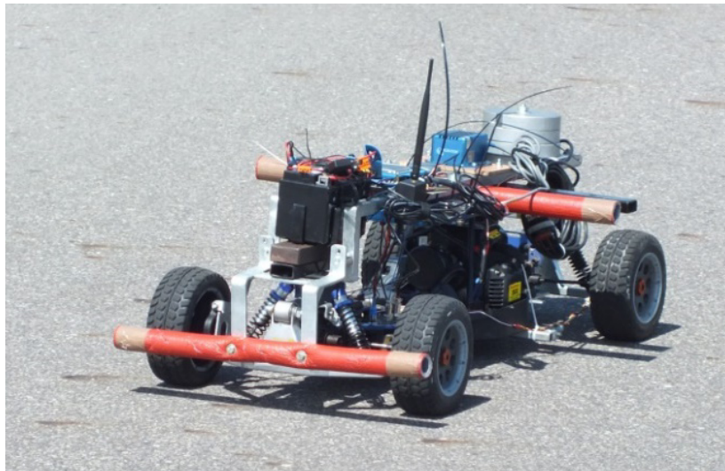
Fig. 6. The vehicle in scale ~1:5 during road tests
