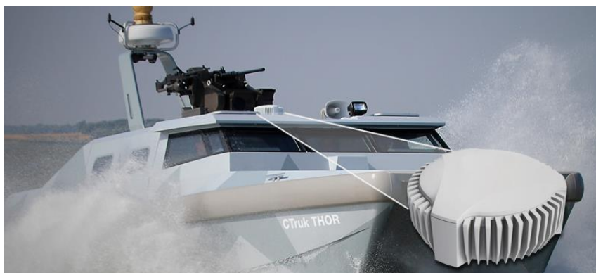
Fig. 5. Utilizing GAJT technology on a vessel [ http://www.novatel.com/products/gnss-antennas/gajt-anti-jam-antennas/gajt-710ms/ (access 26.08.2016)]
