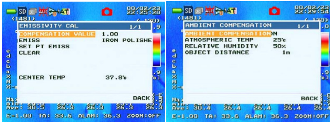
Fig. 2. Emissivity and ambient calibration setting in Thermo Gear G100 [10]
