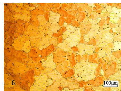
Fig 17. Microstructure CuSi 3 Zn 3 FeMn+0,2%Zr, Stage 6, Time; 37 min, 100x
