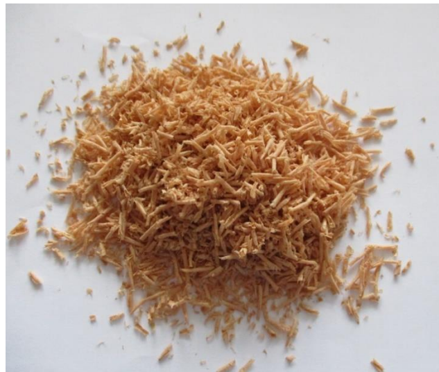
Fig. 2. A look at the chips from milling beech wood at the CNC machining center
