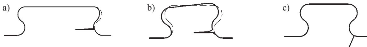
Fig. 3. Failure modes for steel dowel [12]
