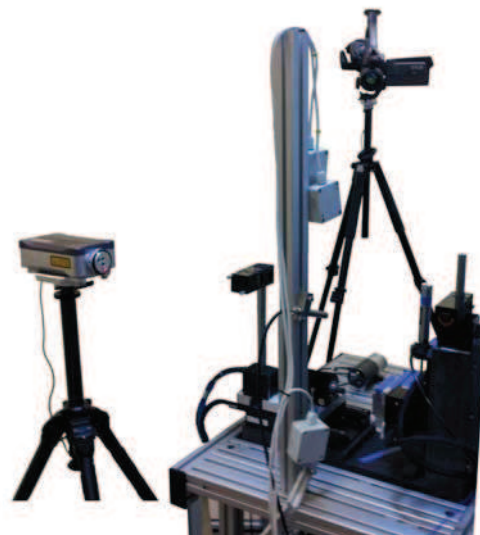
Fig. 12. Photo of the measurement system used to measure thermal deformations of the micro milling machine
