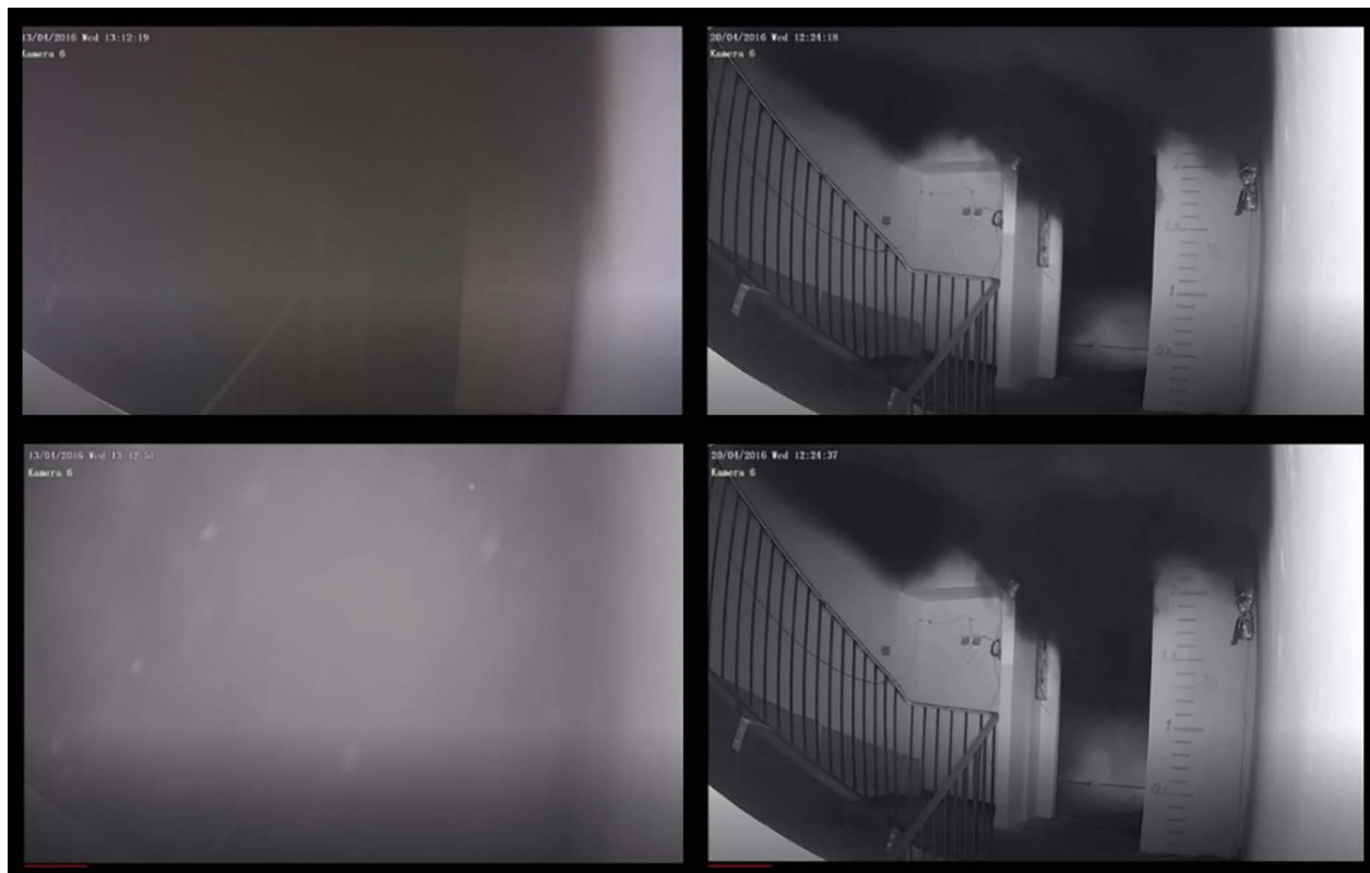
Figure 12. Smoke in the staircase during test 1 (left side) and test 2 (right side), 45 and 75 seconds after opening the door
