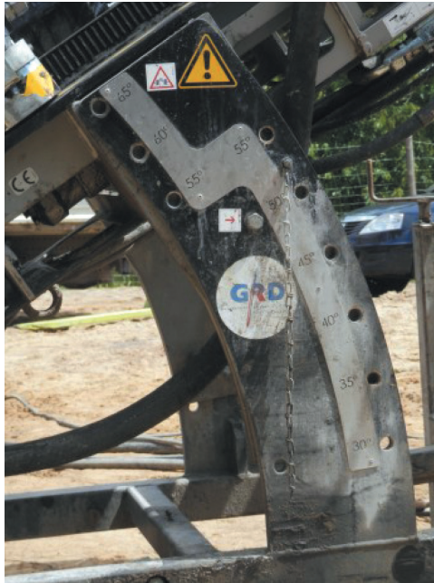
Fig. 5. An angle gauge set to the transporting position [2]
