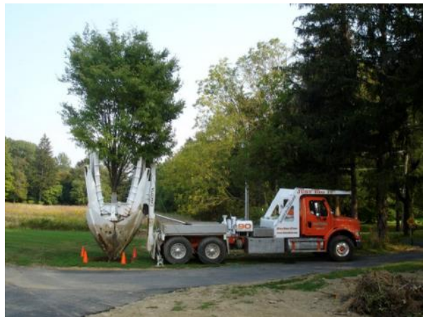
Fig. 20. Tree relocated with a tree transplantation machine. Source: Benckini R. 2017
