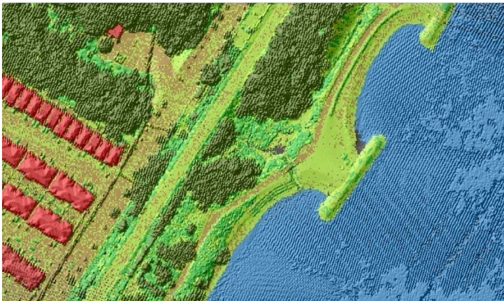
Fig. 10. Shaded DSM (the G channel alone) overlaid with an ALS classification raster (predominant class).
