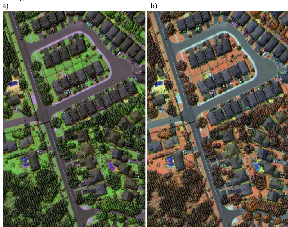
Fig. 8. Shaded DSM overlaid with a colour composition (SWIR, NIR, G (a) and NIR, SWIR, G (b) of multispectral ALS intensity.
