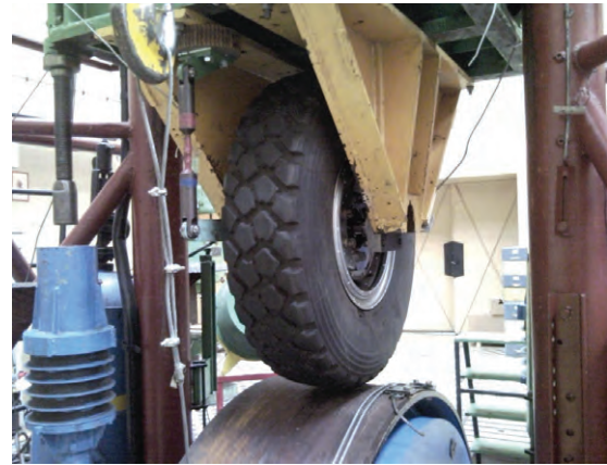
Fig. 8. Młot 3T test rig with automotive brake and wheel mounted during tests
