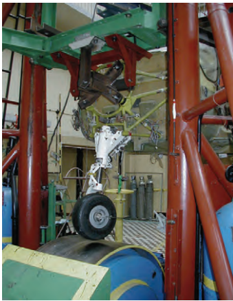
Fig. 7. Młot 3T test rig for full scale brake testing with mounted airplane landing gear
