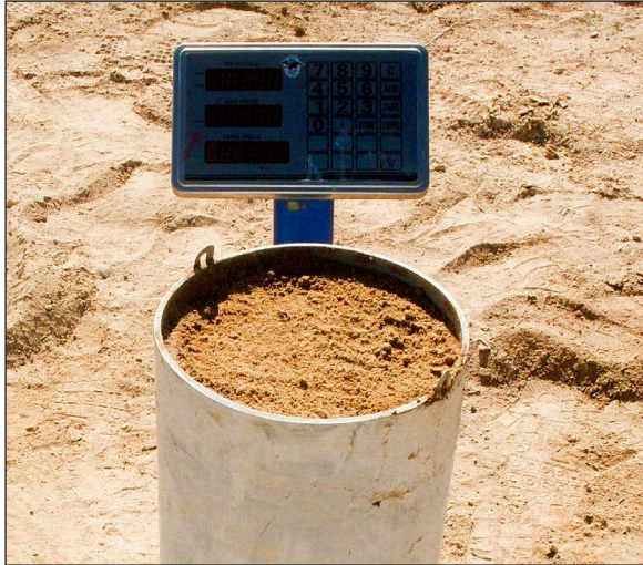
Figure 6. The lysimeter weight was measured using an electronic balance
