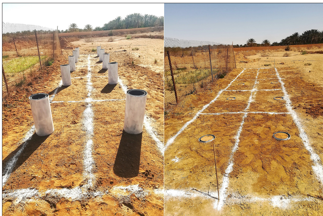
Figure 4. Installation of lysimeters in the INRAA agricultural field
