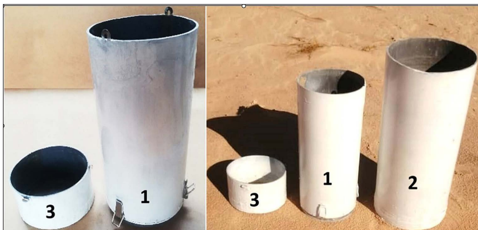
Figure 2. Lysimeter: 1 – inner cylinder (evaporator cylinder), 2 – outer cylinder, 3 – infiltration water collection container
