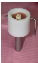
Fig. 2. Restored tooth mounted in the sample container of the dual-axis chewing simulator
