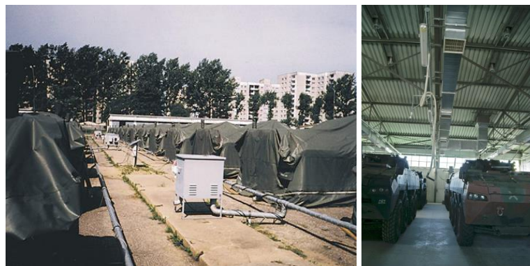
Fig. 7. Equipment stored in dynamically dried covers Source: [Own study].
