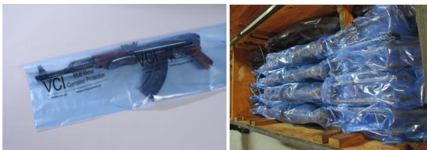
Fig. 3. Examples of weapon protected in the VCI foil and placed in the chest
