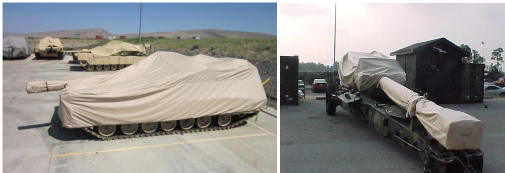
Fig. 5. M1A1 Abrams main battle tank and M198 howitzer protected with ENVELOP cover Source: [Megmar Logistics & Consulting promotional materials].
