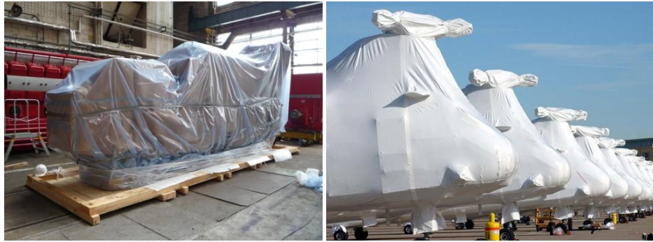
Fig. 4. Examples of the use of VCI foil and paper and VCI heat-shrinkable foil to protect equipment of large dimensions Source: [Maverick promotional materials].
