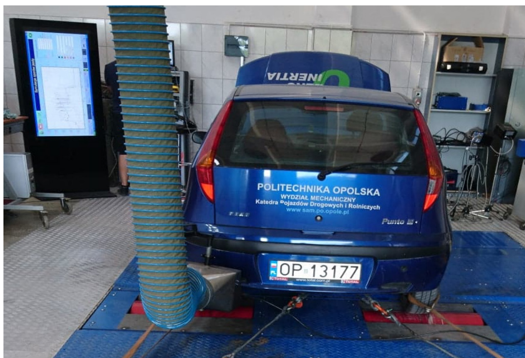
Fig. 1. Test vehicle Fiat Punto II on the measurement stand (chassis dynamometer MAHA MSR 500)
