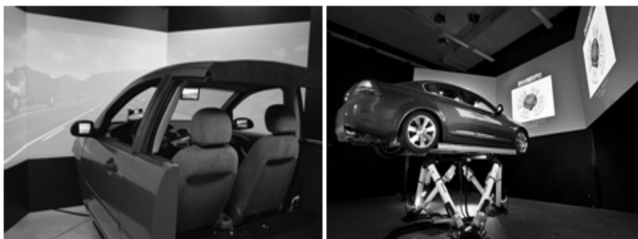
Fig. 2. A model of a static driving simulator (left) [4] and a dynamic driving simulator (right) [5]
