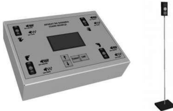
Fig. 1. A model of a device for measuring simple and complex reaction time [2]
