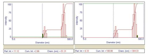
Fig. 3. Histogram of schungite particles distribution according to their sizes after the USD in water during 15 minutes in the presence of NF stabilizer
