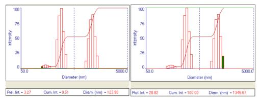
Fig. 1. Histogram of schungite particles distribution according to their sizes after the USD in water during 15 minutes
