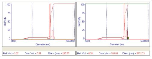
Fig. 2. Histogram of schungite particles distribution according to their sizes after the USD in water during 30 minutes
