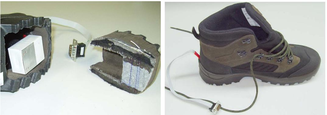
Fig. 7. 16448 module during assembly in the shoe (left) and finished shoe assembly (right) [Popowski, Dąbrowski, 2016]
