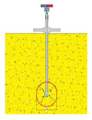
Fig. 2. The way of conducting analysis of the soil gases composition
