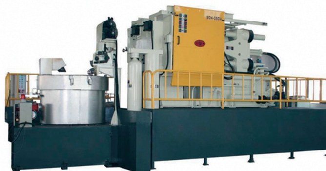
Rys. 10. Hybrydowa maszyna HSC&HPDC o sile zwierania 30 000 kN [20] Fig. 10. A hybrid HSC&HPDC with closing force 30,000 kN [20]
