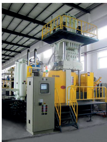
Rys. 11. Hybrydowa maszyna VSC&HPDC o sile zwierania 8000 kN [20] Fig. 11. A hybrid VSC&HPDC machine with closing force 8,000 kN [20]
