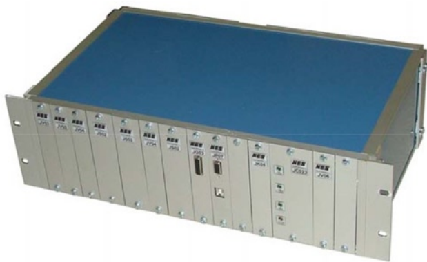
Fig. 2. Control system MORIS RV07 [32]
