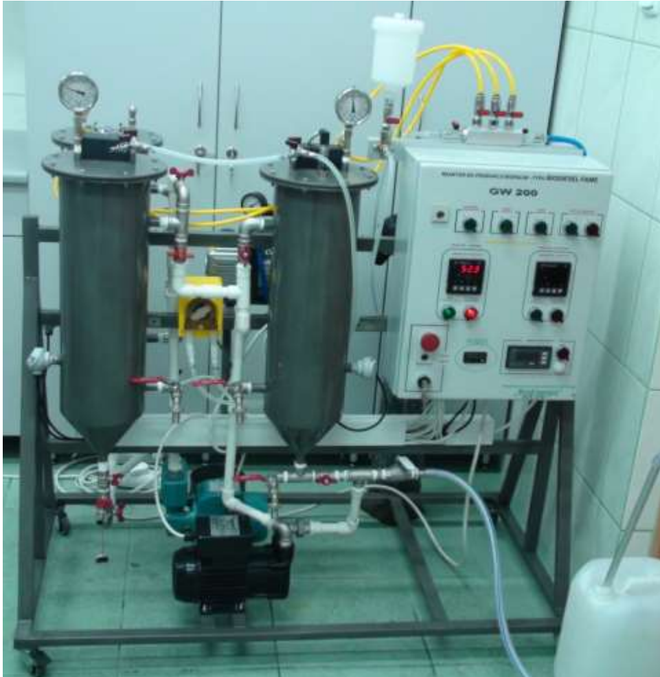
Fig. 2. Reactor GW 200 for production of Biodiesel FAME (FAEE)
