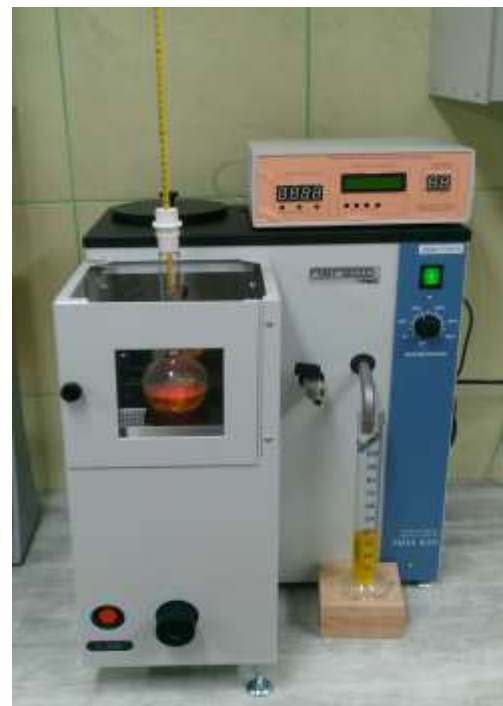
Fig. 3. Photo bench equipped with a distiller HAD 620/1 by Herzog
