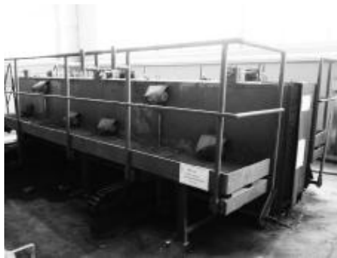
Figure 24. Cassette installation for the production of staircases
