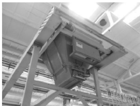
Figure 15. Portal concrete paver
