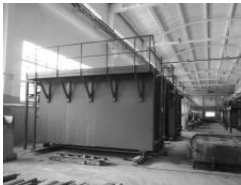
Figure 22. Cassette unit for the production of ventilation units
