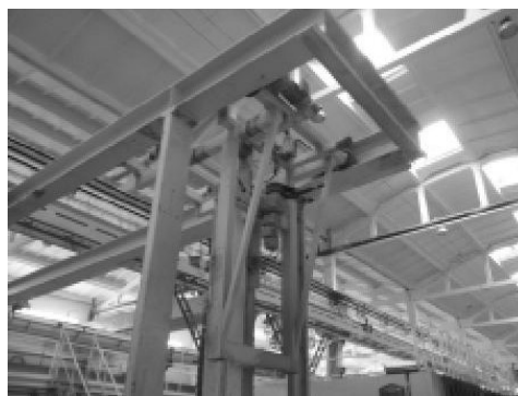
Figure 14. Machine for cleaning and lubrication of cassette units
