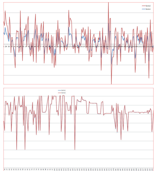
Fig. 14. Comparison of water flows (up) and pressures (down) before and after the water net revitalization performed for 31 pipes
